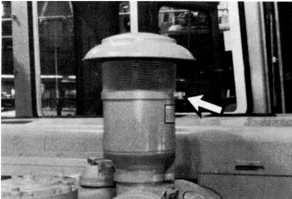
If necessary, loosen the clamp, remove and clean the screen.
